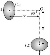
Two very small identical circular loops, (1) and (2), carrying equal currents I are placed vertically (with respect to the plane of the paper) with their geometrical axes perpendicular to each other as shown in the figure. Find the magnitude and direction of the net magnetic field produced at the point O.
